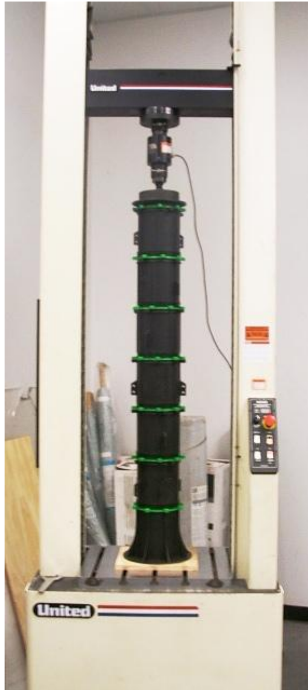
Photograph No.1 52" Pedestal Axial Load Test Set-up
